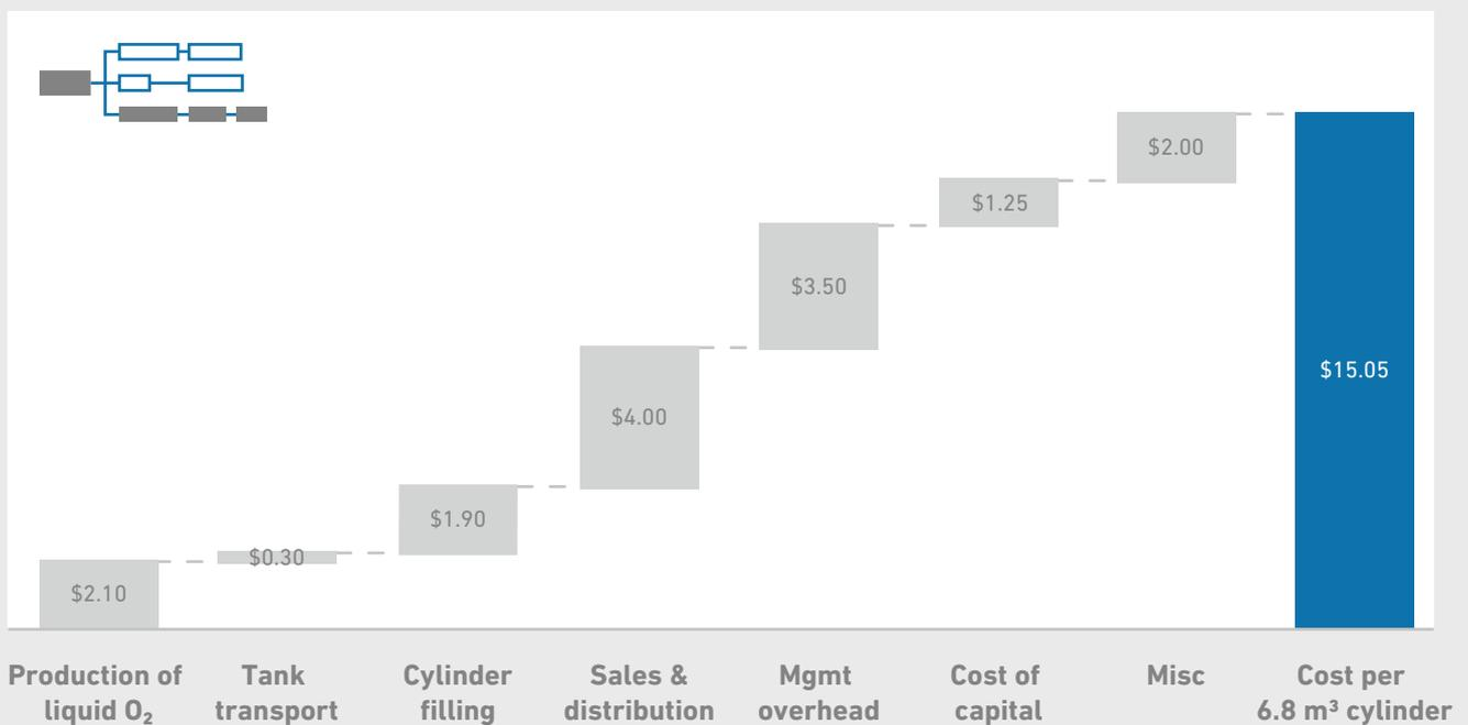
**Exhibit 15:** A hub-and-spoke model with delivery of liquid oxygen to distributed storage filling stations, followed by cylinder filling and final truck delivery to point-of-use, yields a projected TCOD of about \$15.
