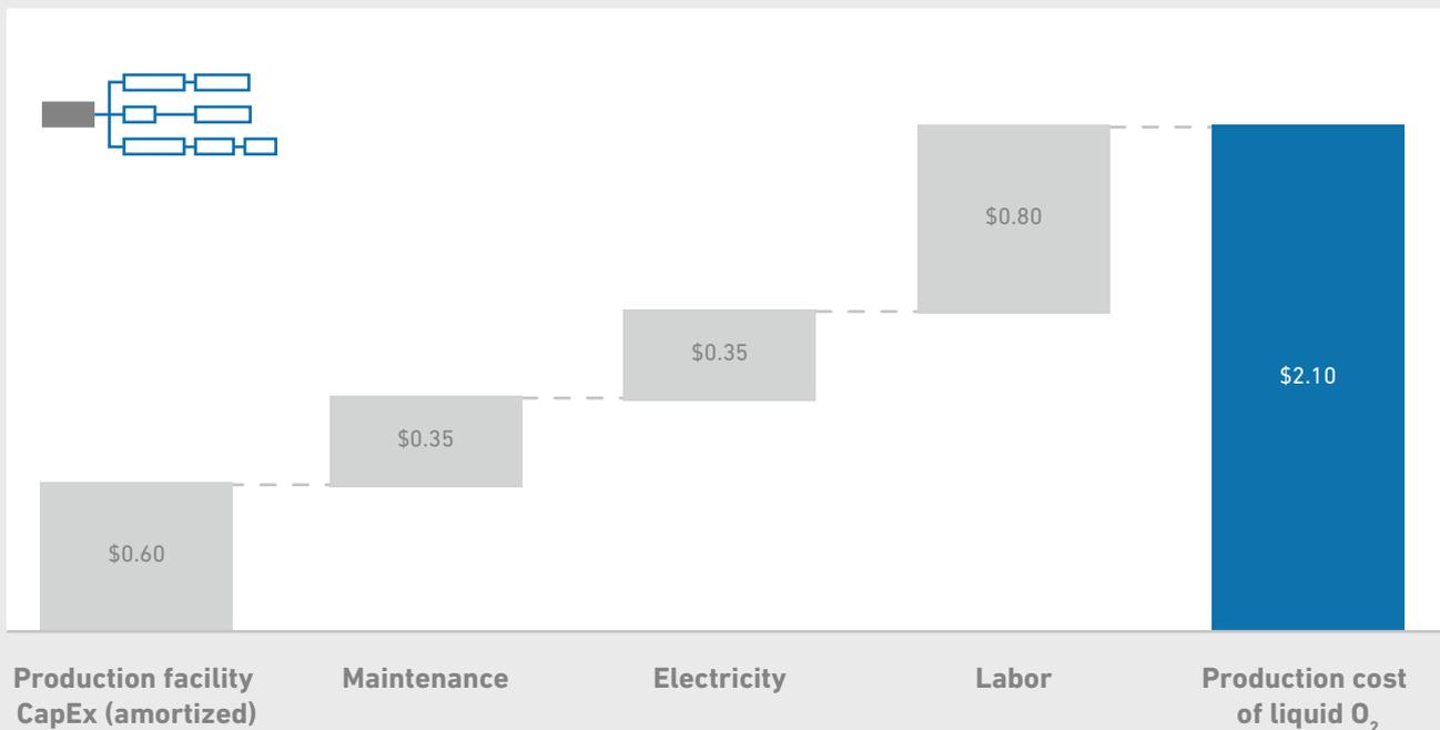
**Exhibit 9:** Production cost of liquid oxygen in Kenya is about \$2.10 for 6.8 m<sup>3</sup> (the volume in one “J” cylinder, but excluding the cost of cylinder filling). Note that amortized CapEx is modeled for small-scale LOX plants located in SSA, with relatively high per-unit capital cost.
