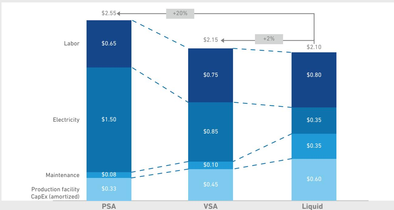
**Exhibit 18:** On a per-unit basis, the production cost of PSA oxygen is 20% higher than that of LOX and VSA. The largest driver of cost is electricity. Note that this only describes production cost, not the total cost of delivery to patients (which is much higher). Also, per-unit CapEx for PSA and VSA compare favorably to LOX because we use the example of the smaller LOX plants common in SSA.
